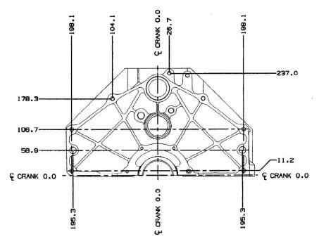
Figure 3.3.4.3 Rear Face of Block
